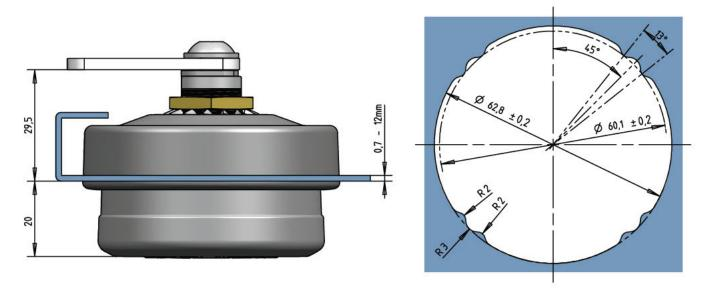
2. Recessed installation in wooden doors using special milling and optional installation shell (Specify when ordering)
