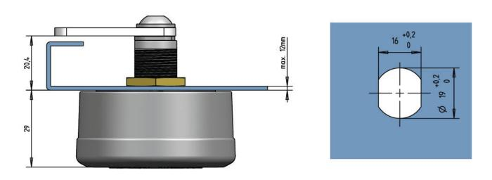
2. Fastening in wooden doors by means of cup drilling and optional anti-rotation bolt (Specify when ordering)
